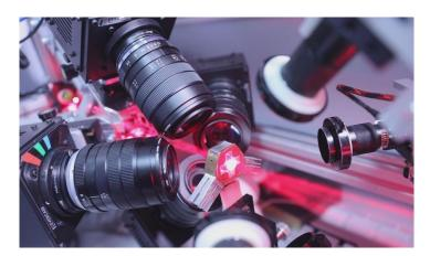
**Fig2.** The setup designed and constructed by Sergey Farisenkov for high-speed recording of the free flight of microinsects under infrared LED and laser illumination using four synchronized cameras. Photo from the archive of the Department of Entomology, Faculty of Biology, Lomonosov Moscow State University
